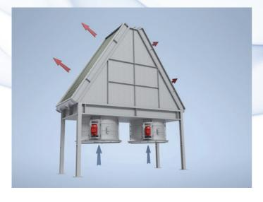
In cases of limited space, systems are can be installed in an A-frame roof configuration. The fans are positioned in a forced arrangement.
