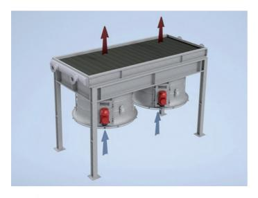
The most common design of air coolers is the horizontal configuration with forced fans beneath the heat exchange bundles. This arrangement provides easy access to the fan drives for maintenance purposes.
