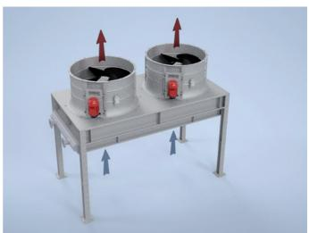
The induced arrangement of fans, positioned above the heat echanger bundles, ensures a very uniform flow over the heat transfer surface. The shading of the heat exchange bundles provides protection against intense sun radiation.
