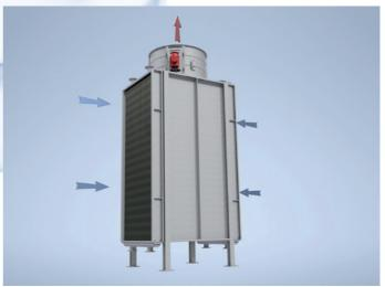
Vertical configuration systems are used in situations with limited space. In a vertical airflow arrangement, the fans are positioned in induced mode. Especially in smaller systems the fans can be arranged with horizontal airflow (forced or induced).
